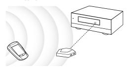
Therefore, the RF Receiver has to be placed near the device you're operating with the RF Receiver's sending eye pointed to the device. Your devices will always receive IR signals either directly from the remote controller or from the RF Receiver.
